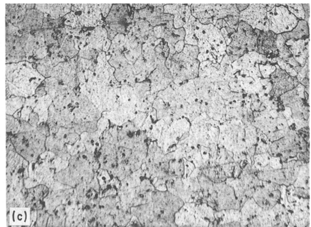
Figure 5 Photomicrographs of sintered iron compacts with different pore volume fraction p (a) sample no. 20, p = 0.216 ; (b) sample no. 16, p = 0.121 ; (c) sample no. 18, p = 0.03 .
